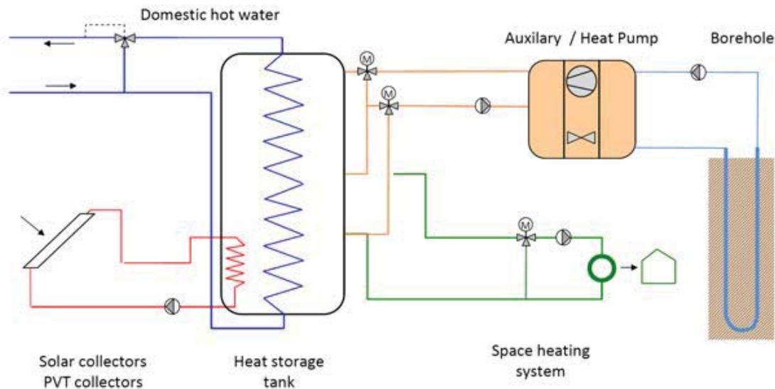
Fig. 2 Reference solar heat pump system scheme
