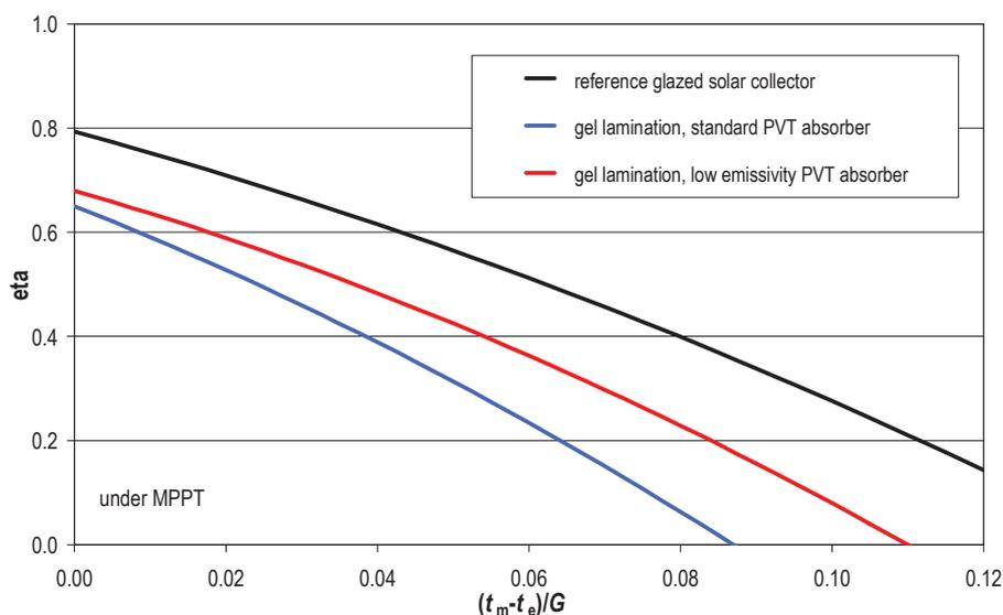
Fig. 1 Efficiency characteristics for different concepts of solar PVT collectors compared with standard glazed solar thermal collector (reference)
