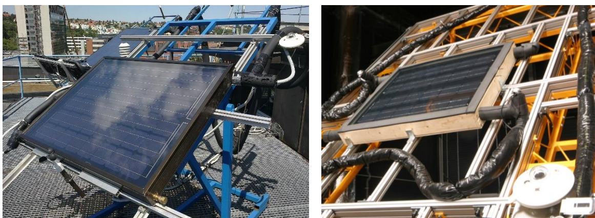
Figure 6: Glazed nonselective PVT collector at outdoor testing, glazed selective PVT collector at indoor testing.
