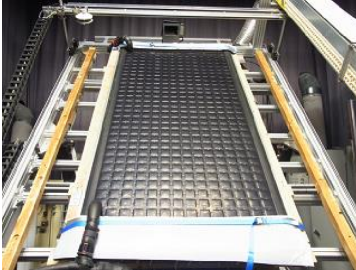
Figure 3: Test collector exposed under the artificial sky at the SPF solar institute.
