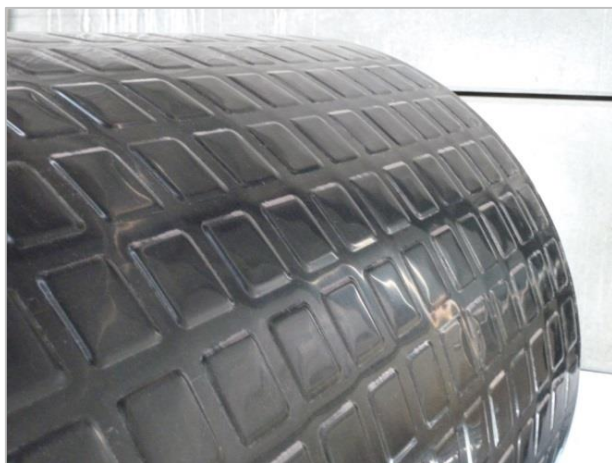
Figure 2: Ferritic stainless steel coil with new selective paint (after stamping of cushions).
