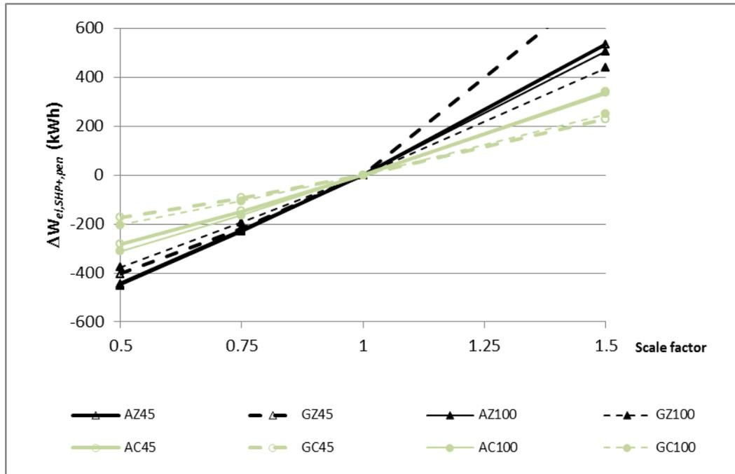
Fig. 6 Change in system electricity use as function of the DHW discharge energy.
