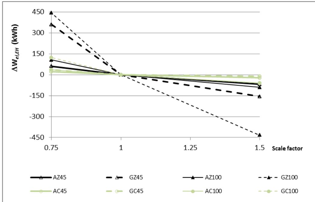
Fig 12 Change in the use of auxiliary electrical heater as function of the size of heat pump.
