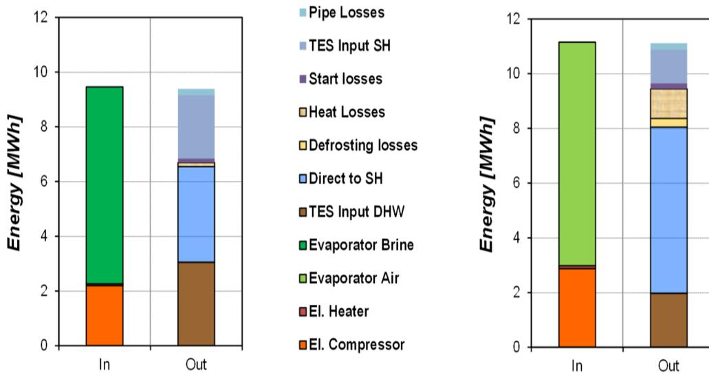
Fig. 4 Heat balance for heat pump in the two reference systems. GSHP (left) and ASHP (right).
