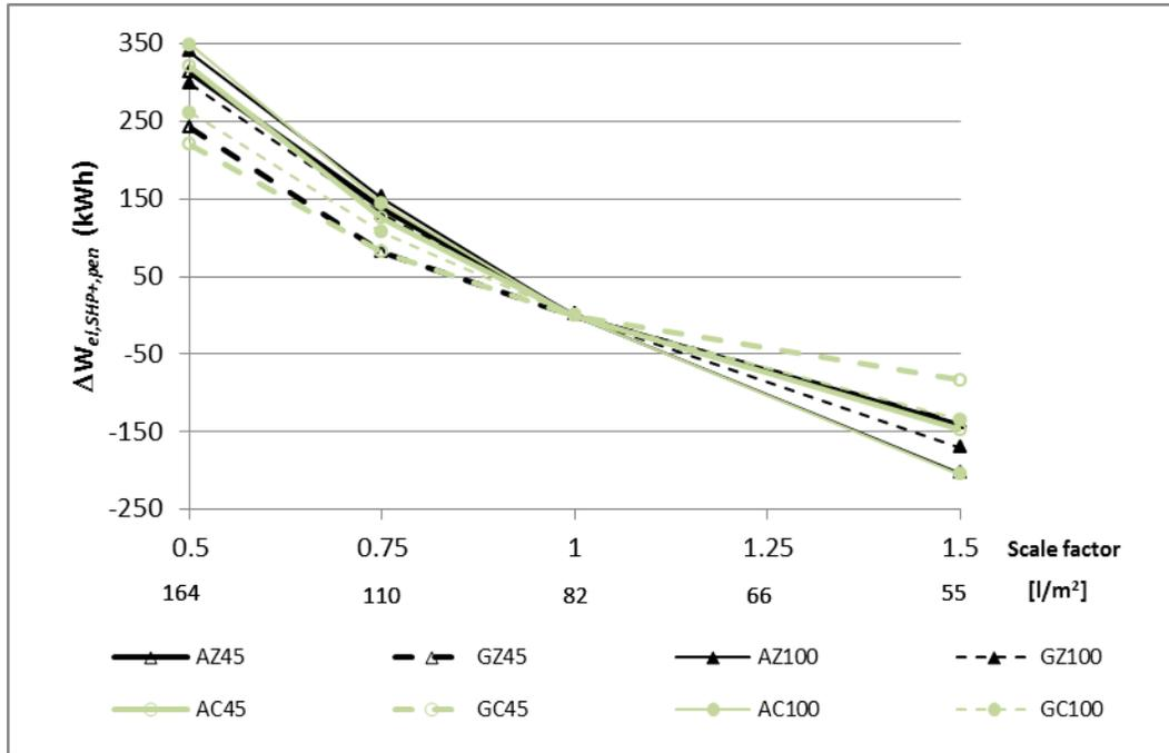
Fig. 7 Change in system electricity use as function of the size of the collector.
