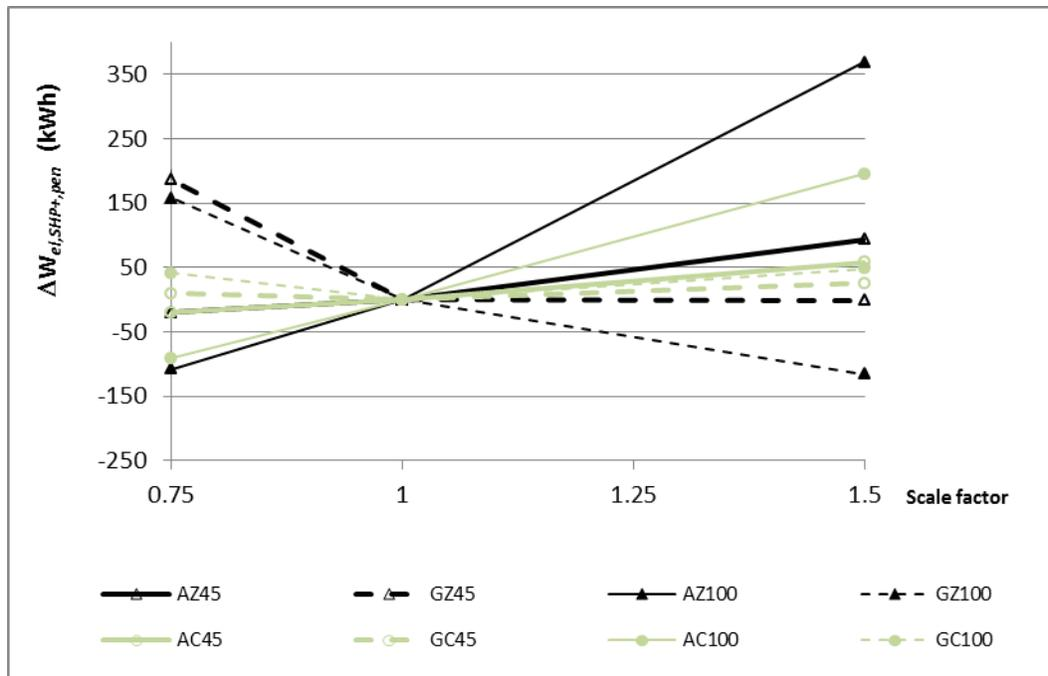
Fig. 10 Change in system electricity use as function of the size of heat pump.
