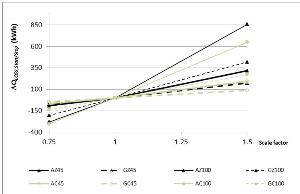
Fig. 11 Change in heat pump start/stop losses as function of the size of heat pump.
