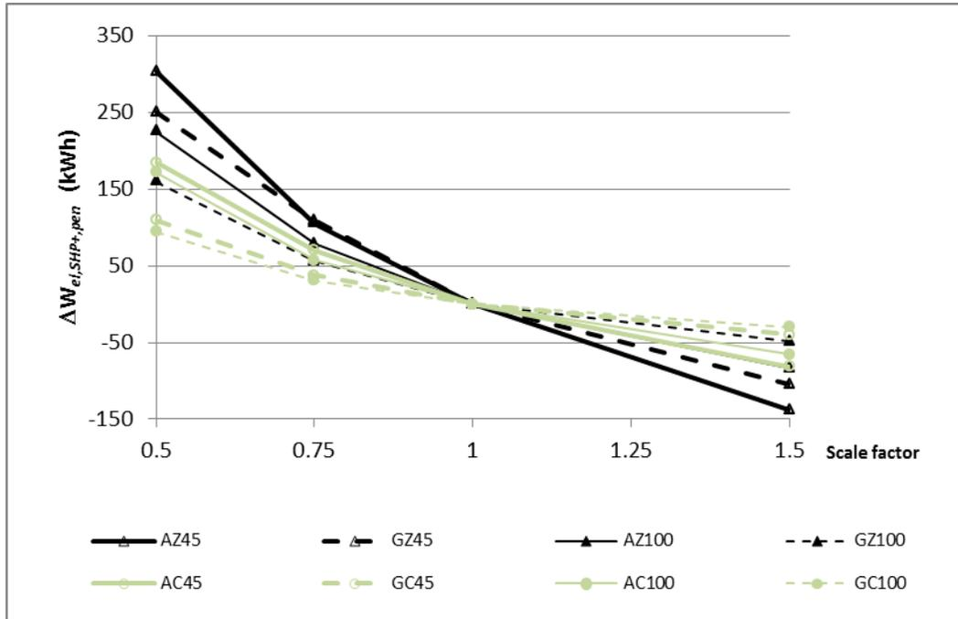
Fig. 9 Change in system electricity use as function of UA-value of DHW heat exchanger.
