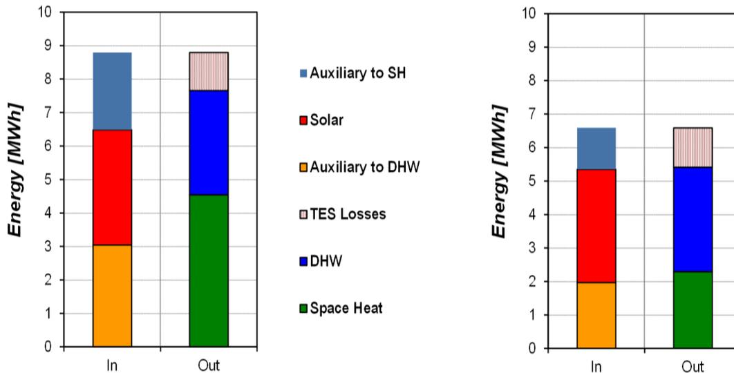
Fig. 3 Heat input and output from the stores in the two reference systems. GSHP (left) and ASHP (right).
