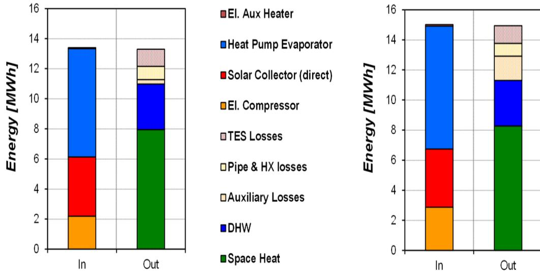
Fig. 2 Overall system results for the two reference systems (only thermally active parts). GSHP (left) and ASHP (right).
