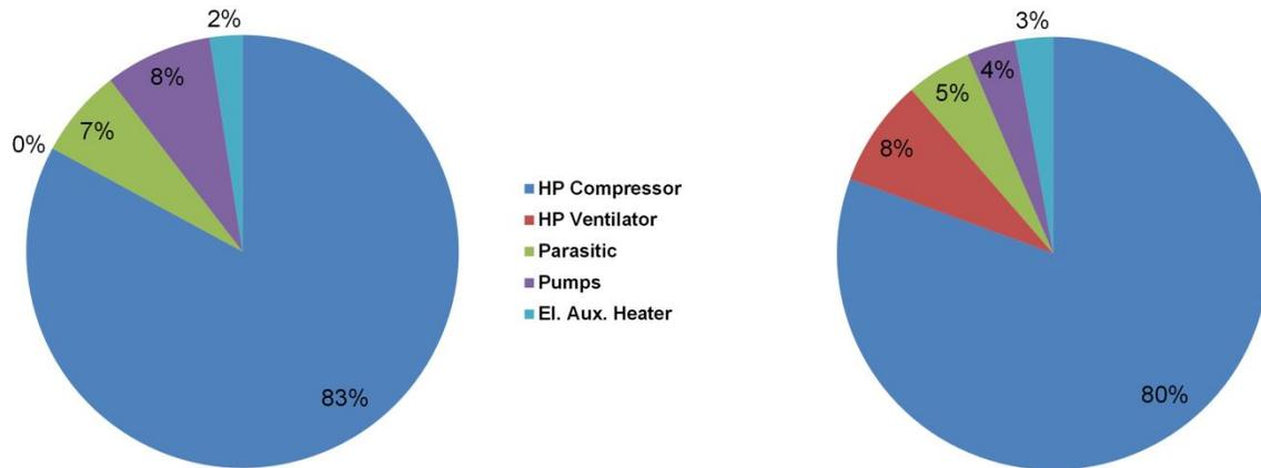
Fig. 5 Electricity use in the two reference systems. GSHP (left) and ASHP (right).
