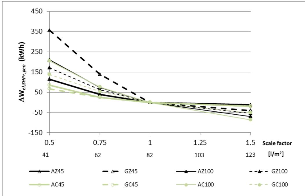
Fig. 8 Change in system electricity use as function of the size of the tank volume.
